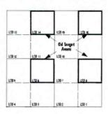
Together, the oil and gas target areas overlap and form a **common target area**, as shown in the shaded portions of the figure below. Many companies prefer to drill the common target area if there is a chance to encounter both oil and gas.
